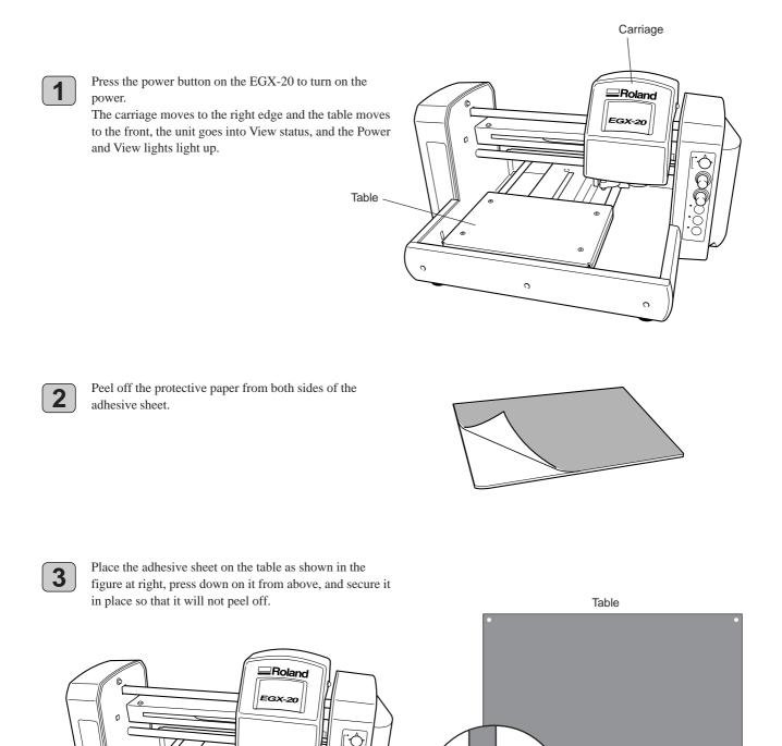
There are holes at the four corners of the table. Align the corner of the adhesive sheet with the lower-left hole.
